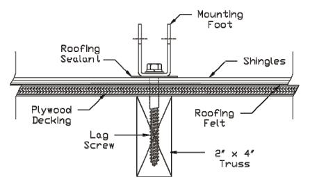
Figure: Lag Bolt Mounting
