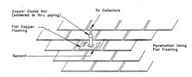
Figure: Piping through roof
