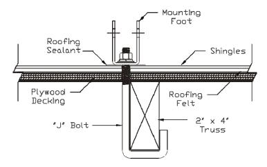
Figure: J-Bolt Mounting
