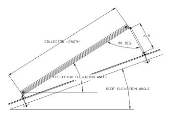
Note: The Tilt mounting Struts should be cut to length to provide the required collector elevation angle as described in the following section.
