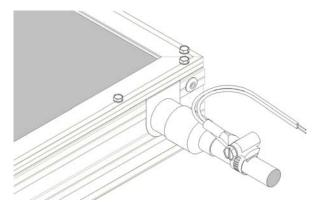
Figure: Installing the Collector Sensor
