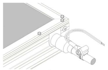
Figure: Installing the Collector Sensor
