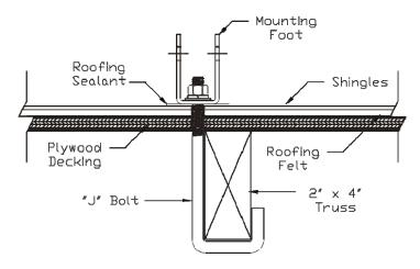
Figure: J-Bolt Mounting
