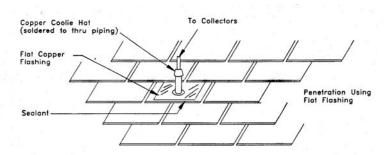
Figure: Piping through roof
