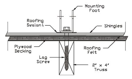
Figure: Lag Bolt Mounting
