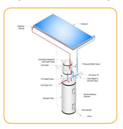
solar collector loop, simultaneously, water is circulated from the hot water tank through the finned coil heat exchanger inside the reservoir.
