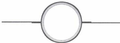
The mechanical joint is the simplest construction, but it offers comparatively poor thermal conductivity. To overcome this problem, the contact area must be large and the joint must be uniformly tight (requiring wrapping the fin around most or all of the tube). However, when the joint loosens with age and thermal cycling and develops a gap, or when the contacting surfaces corrode, the heat transfer capability will be greatly reduced.
