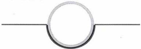
Although solder or adhesive bonding avoids certain of the problems of mechanical joining, low thermal conductivity remains a problem. To provide sufficient heat flow from fin to tube, both a large contact area and a thin, continuous layer of the bonding agent are necessary, and this bonding agent can deteriorate with aging and thermal cycling.
