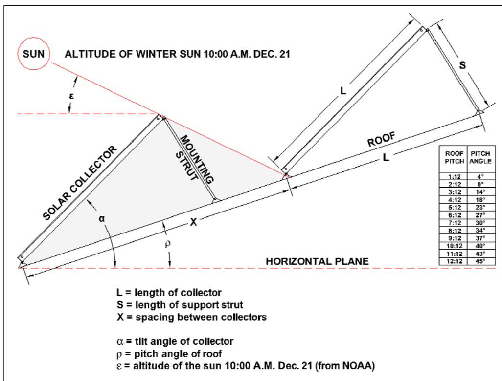
To calculate the length of the support strut use the formula as follows:
